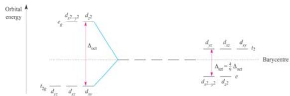
**Fig. 21.8** Crystal field splitting diagrams for octahedral (left-hand side) and tetrahedral (right-hand side) fields. The splittings are referred to a common barycentre.
